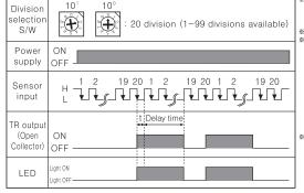
When selecting Re-start mode while operating, cut off the power and turn it on again. ×Delay Time: Approx. 30ms
